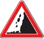
Risk of falling rocks or presence of fallen stones on the road
