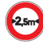
Road closure to the vehicles whose width is higher than the number indicated
