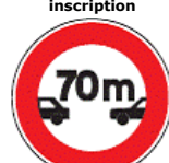
Prohibition with the vehicles to circulate without maintaining between them an interval at least equal to the number indicated
