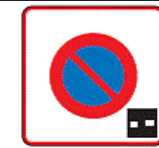
Entry of a zone with parking at limited duration
