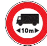
Road closure to the vehicles of which the length is greater than that indicated by the figure
